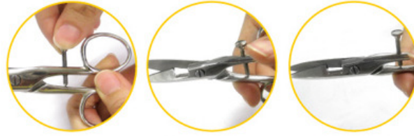
1. set the gauge 2. for small buttonhole 3. for large buttonhole
